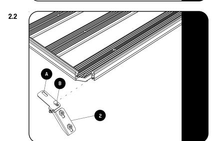
Slide 4 loosely assembled Wind Fairing Adjustable Brackets (Item 2) into the bottom channel using either slot A or B as shown in Figure 2.2.
