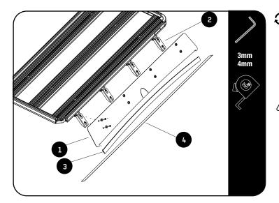
Remove the M5x16 Countersink Screws & M5 Finishing Washers from the bracket.
