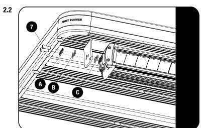
Fit the LED light to the brackets as shown, using the M6 x 16 Button Head Bolts (Item 7) and fasteners supplied with the light .
