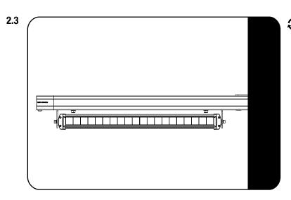
Fully tighten all the fasteners.
