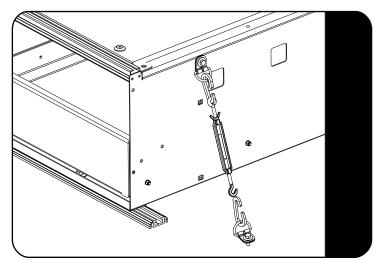
Connect a turn Buckle and C-Hook (Item 12) to each of the D-Rings (Item 4) assembled to the drawer system in step 2.3
