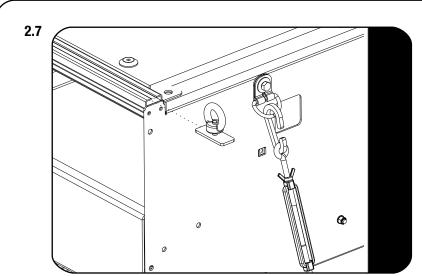
Should you wish to use the Eye Nut assemblies from step 2.2 as tie down points, they can be slid into any of the 3 top extrusions as shown and tighten in the requierd position.
