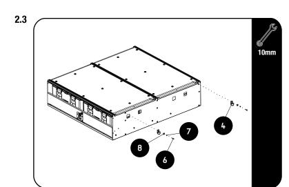
Assemble two D-Rings (Item 4) to either side of the Drawer as shown using the M6 x 20 Hex Bolts, M6 x 19 Flat Washer and M6 Spring Washer as shown (Item 6,7 & 8).
