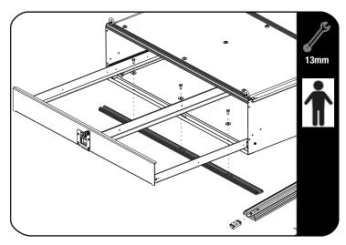
Slide the 3 channel Nuts (Item 16)into the Track(Item 17).Place the Track under the Front cross strap of the Drawer.Line the 3 channel nuts inside the track up with the mounting holes in the cross strap as shown.
