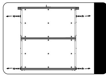
With the Turn Buckles and C-Hooks in position, work out how best to secure the "hook end" of the turn Buckle to the vehicle.
