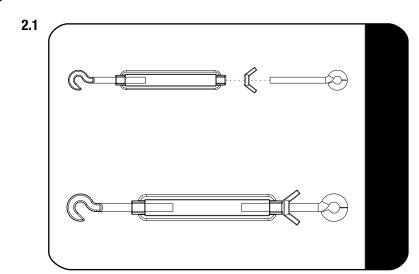
Loosen the round end of the Turn Bucle (Item 5). Screw a M6 Wing Nut (Item 3) on to each round end of the Turn Bucle. Reassemble the Turn Bucle as shown. Do this with all 4 turn Bucles.
