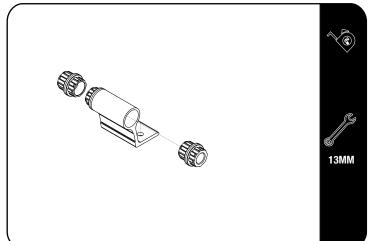
Choose which Thru Axle Insert is suitable for your bike and assemble one pair as shown.
