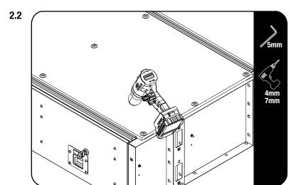
Remove the Fridge Slide and Drill a 7mm hole through the wood on each of your markings. Loosen and remove the deck.
