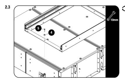
Secure the Deck back onto the drawer system. Place the fridge Slide (Item 1) back into position and secure using M6 x 20 Hex Bolts and M6 x 19 x 1 Flat Washers (Items 4 & 5).
